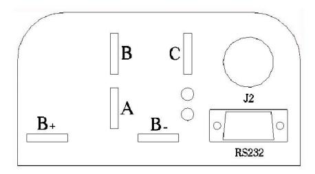
Figure 3: Brushless motor controller front panel
